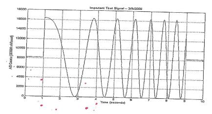
Below is a plot of the same data file having being read in as unsigned integers on a big endian machine. The data is good! It is the same as above! All that has changed is the endianness of the machine that read the data.
