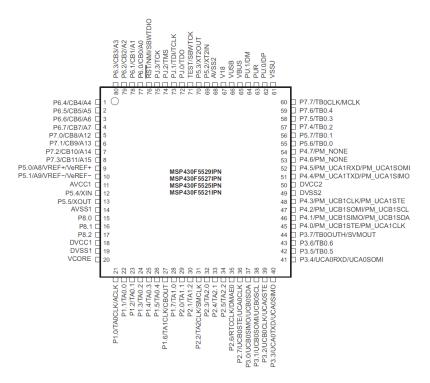
In order to maximize the usage of physical pins, most physical pins (also called "package pins") are shared between multiple device functions.
