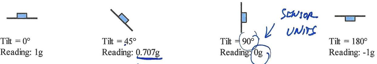
An older version of the ECE2049 lab boards had a ADXL335 3-axis accelerometer, which provides three output signals  $X_{out}$ ,  $Y_{out}$ , and  $Z_{out}$  as analog outputs with output voltages that correspond to the acceleration along each axis. For this problem, we only need to read the output on the z-axis, which provides enough information to measure tilt (as shown in the examples).
