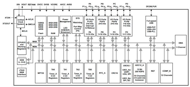
Note the lines connecting all of the peripherals: this is the memory bus!
