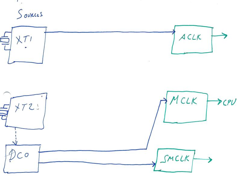
In addition, you also need to configure some parameters for the sources (like the DCO), and the signals (like clock dividers).
