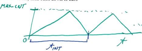
In each mode, most timers (like those on the MSP430) will trigger an interrupt when the count transitions back to 0.
