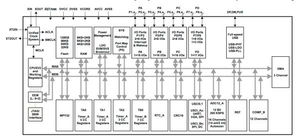
MSP430s have two main types of timers, Timer A, and Timer B; both types function in very similar ways, but have some subtle differences. Each chip can have multiple Timer A's and B's, as shown in the block diagram.
